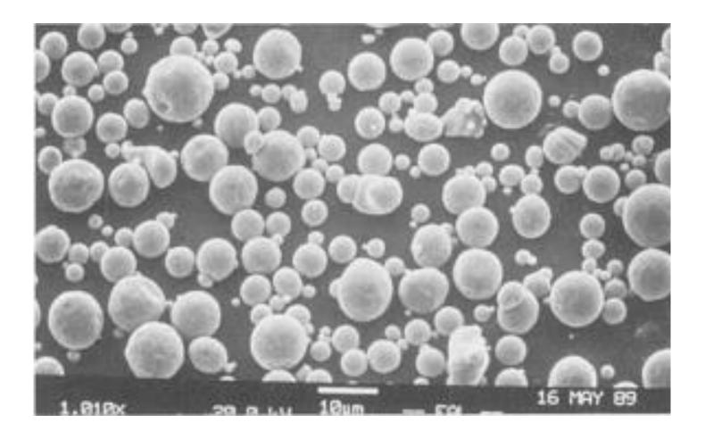
**Figure:** Scanning electron microscopy of 316L stainless steel gas-atomized powder.
